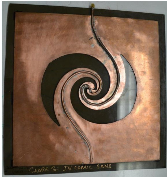
Figure 1: A photo of the completed antenna
